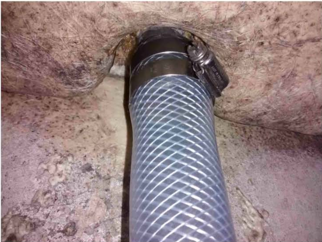
The hose where it connects to the remaining ruddertube.
