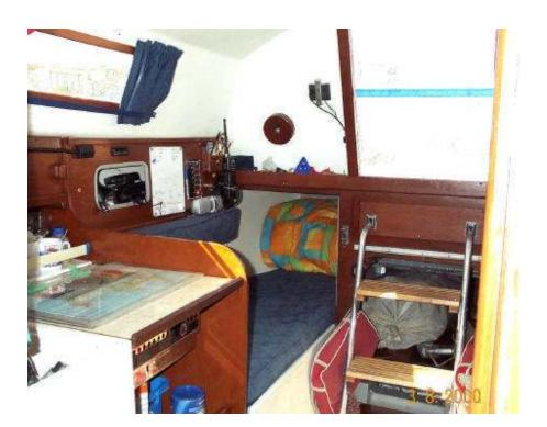
Down below, two settee berths run partially under the cockpit seats – the starboard one making a good sea berth. Forward of this is the galley area with moulded sink and room for a full size cooker or gimballed two-burner hob with stowage under if preferred. Heads compartment is on the port side with a small hanging locker opposite.
