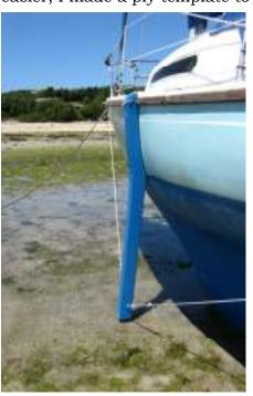
water line splayed the legs outwards. When happy with the shape I got my local joinery shop to cut them out of a 4in thick Iroko plank, having got the rough shape I worked on them to get them fit for painting.
