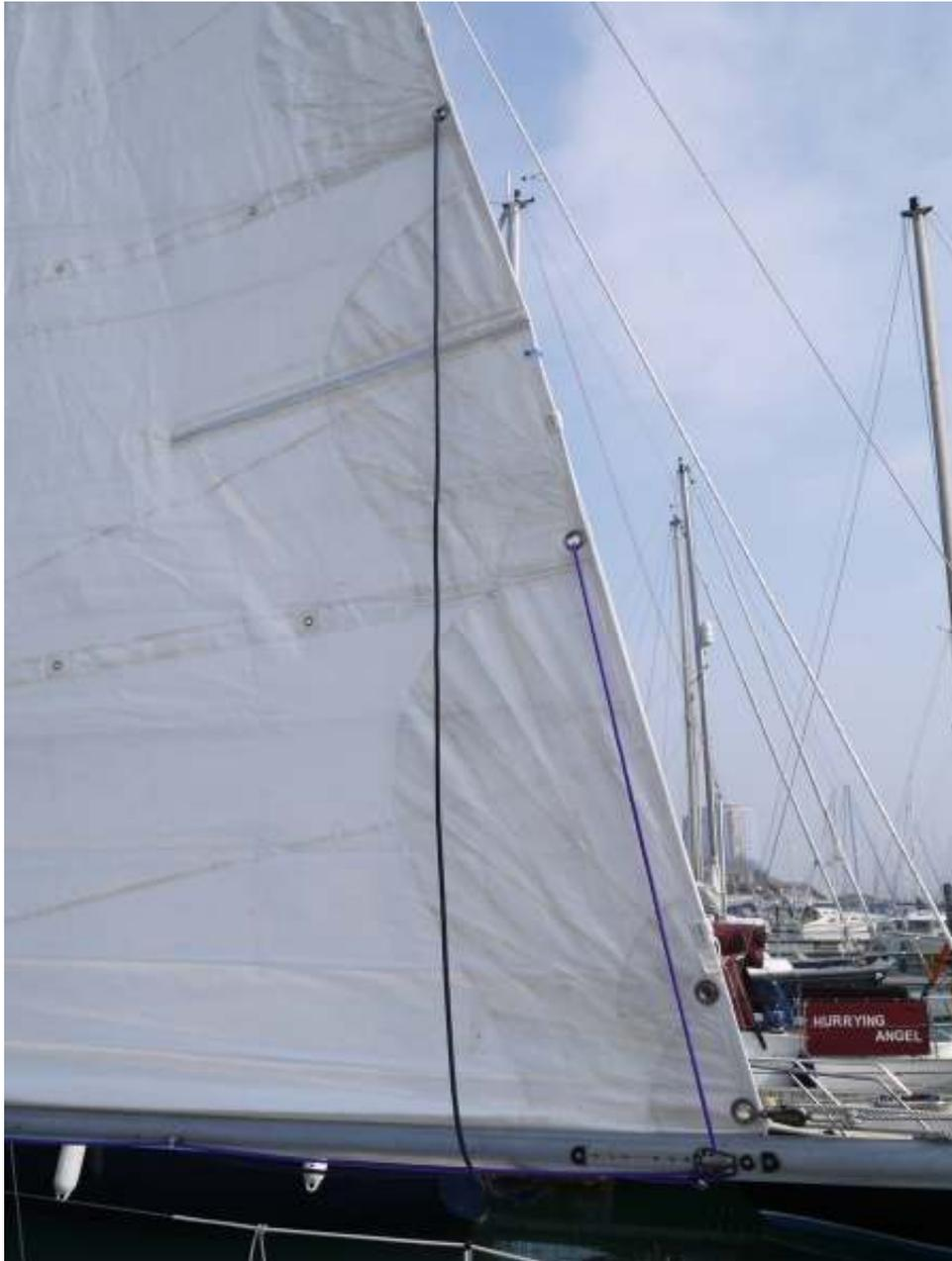
*No1 reefing slide on the boom; both reefing lines rigged.*
