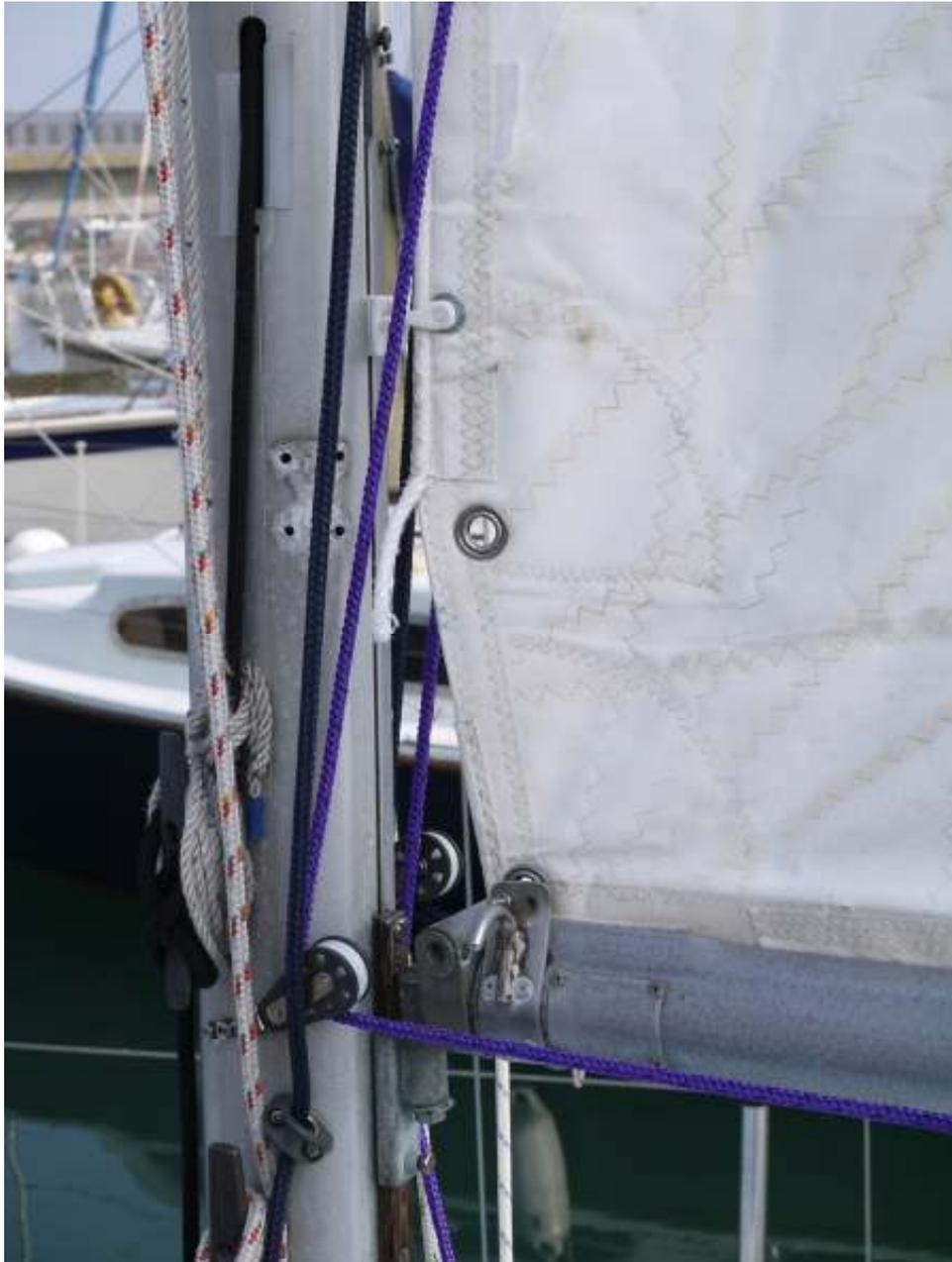
*Left/top (port side) – the tang block for No1 reefing line above the bulls eye for No2 reefing line. In the background you can see the tang block for No2 reefing line (stbd side). The No1 bulls eye is out of view but you can see the No1 reefing line leading downwards to the upright block.*
